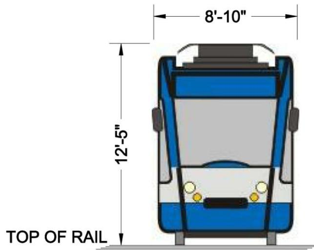
**Figure 2: Typical LRT Dimensions (overhead catenary wires not shown or included in the dimensions)**
