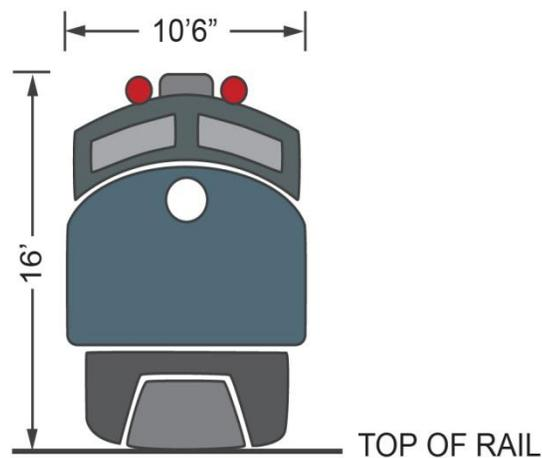
**Figure 3: Typical CRT Dimensions**
