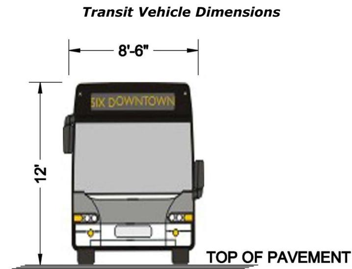
**Figure 1: Typical BRT Dimensions**
