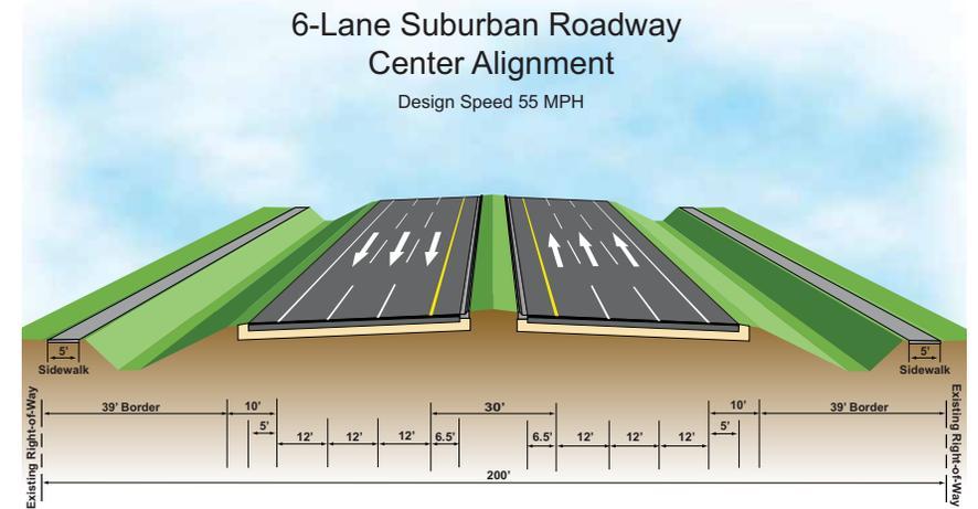
This highway cross-section is proposed by Florida DOT for SR 82. SOURCE: [www.sr82pde.com/SR%2082%20Preferred%20Typical%20Section.pdf](http://www.sr82pde.com/SR%2082%20Preferred%20Typical%20Section.pdf)
