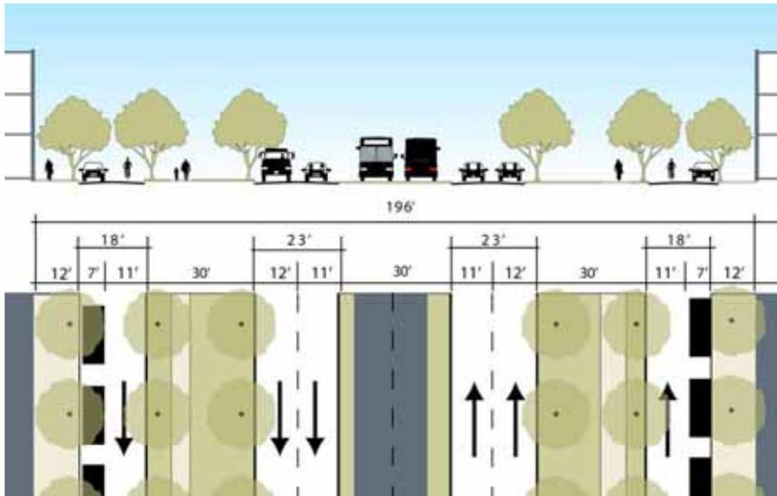
This alternative cross-section of SR 82 includes through lanes for cars, dedicated lanes for bus rapid transit (or any other form of transit), wide side medians for walking and biking paths, and local access lanes to support local traffic.
