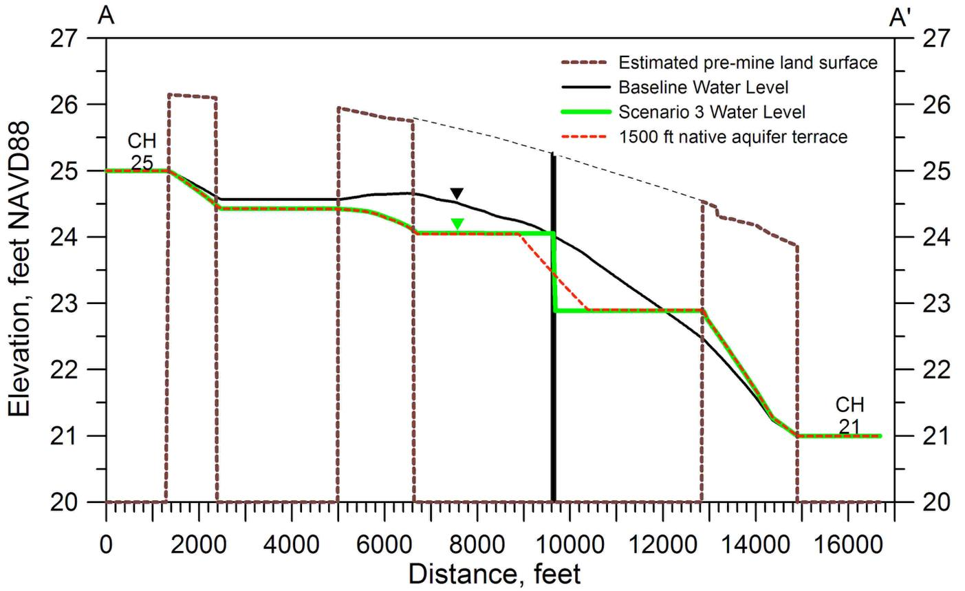
Figure 4.15: Profile of Groundwater Levels Comparing 1,500-foot-wide Native Aquifer Terrace versus Slurry Wall
