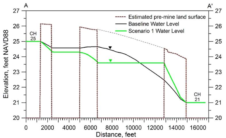
Figure 4.5: Simulated Contours and Water Level Profiles of Groundwater Elevation for Scenario 1
