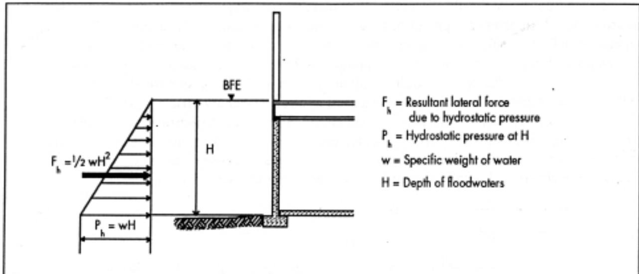
Figure 5. Lateral Hydrostatic Force and Pressure
