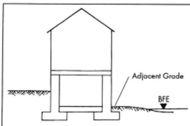
Figure 2. Compliant Grading for a Walkout Basement
