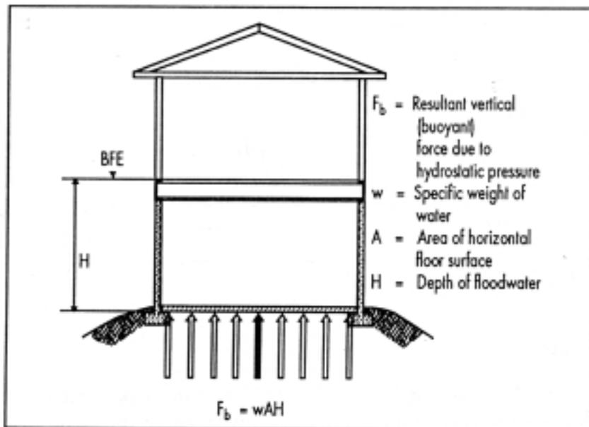
Figure 6. Buoyancy Force
