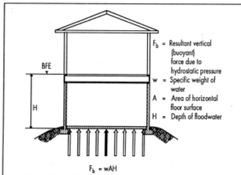
Figure 6. Buoyancy Force
