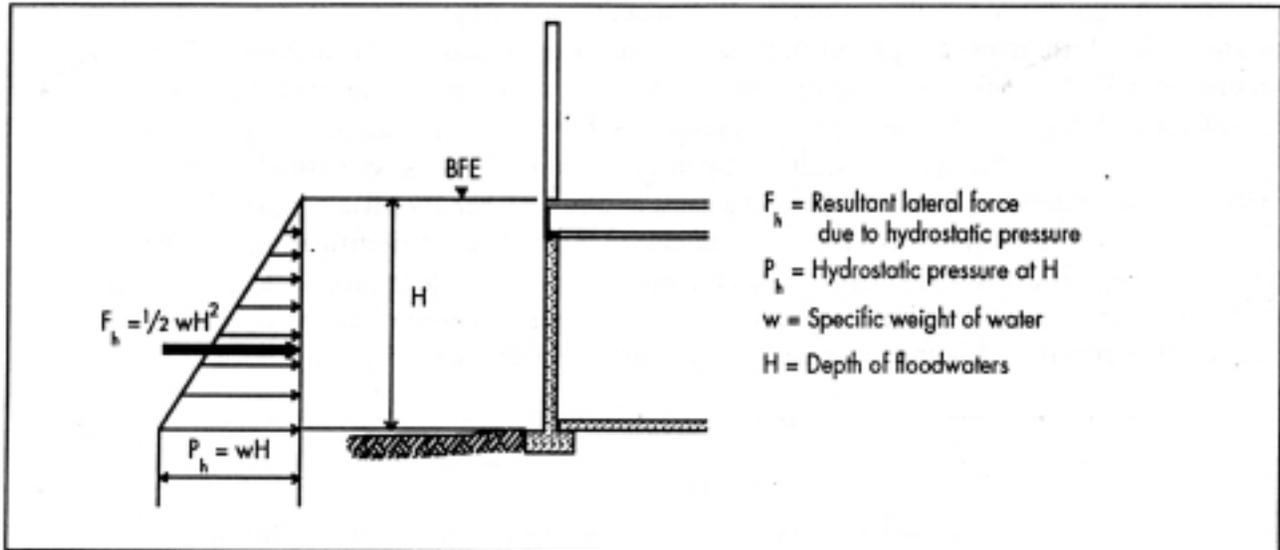
Figure 5. Lateral Hydrostatic Force and Pressure
