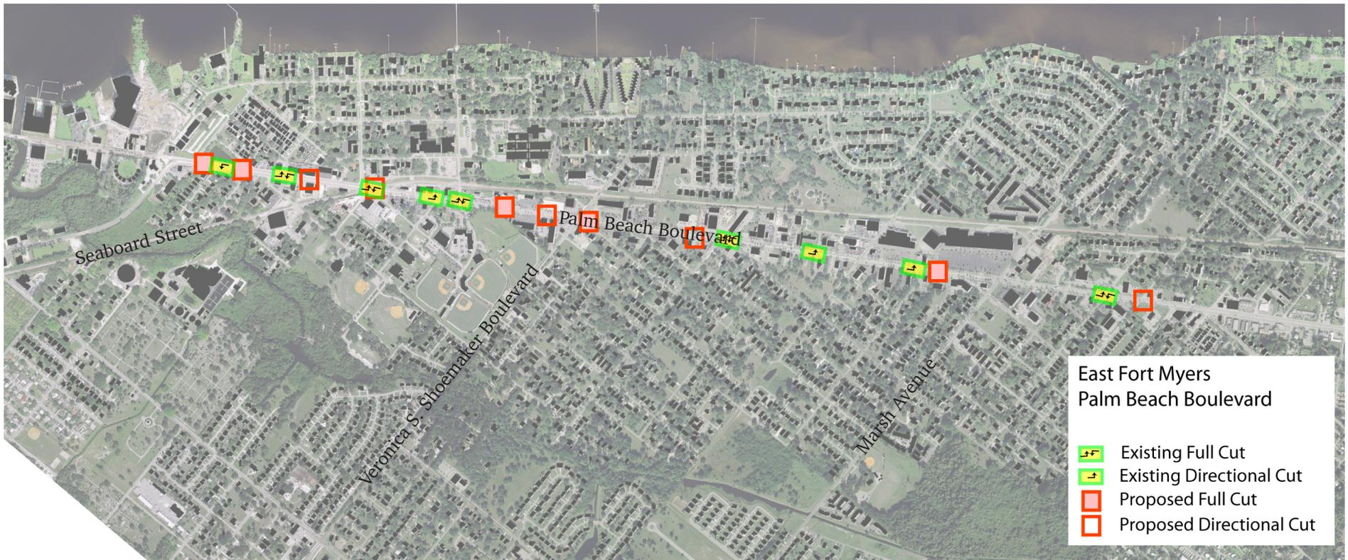
Figure 5.3: Current and Proposed Median Openings along Palm Beach Boulevard. The added median openings are needed as noted above from east to west; a directional opening at Prospect Avenue would serve longer trips on the north side due to the rail crossing.
