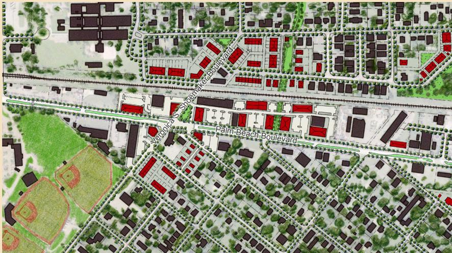
**Step 2.** Infill and redevelopment continue to occur. Buildings are built closer to the edge of the sidewalk. Surface parking lots are repositioned to the rear and side of buildings rather than along the front.
