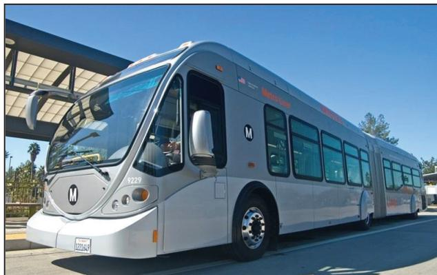
BRT relies on a combination of limited-stop service and advanced technology to help speed up travel times and improve service reliability. BRT service can be designed to operate in exclusive transitways or busways, such as the SGLR corridor, as well as in mixed-traffic on expressways or arterial streets.
