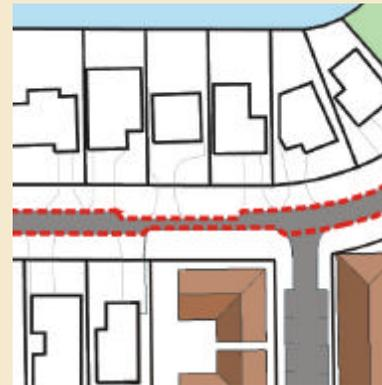
Plan view of the proposed neck down located along 107th Avenue- the red dashed line marks the edge of pavement.
